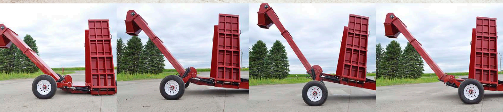
OPERATING POSITION TO TRANSPORT POSITION WITH A PUSH OF A BUTTON
