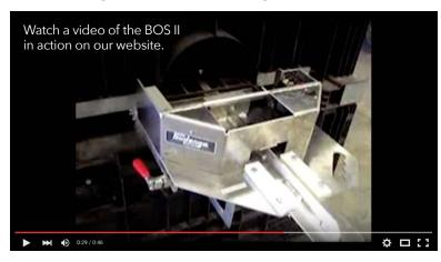
With almost 50 lbs of linear pulling force, the electric gate opening actuator opens and closes gates even when they are under load or flowing seed.
