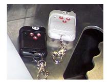
Using the small hand-held remote control, seed boxes are unloaded into planters, drills, etc. from the forklift driver's seat
