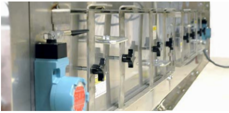
LARGE ACCESS DOORS The large access doors allow for easy access for rotating drum inspection.
