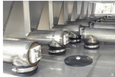
MICRO HOPPER DISCHARGE UHMW bearing on the micro hopper discharge end provides lubrication free and maintenance free operation.
