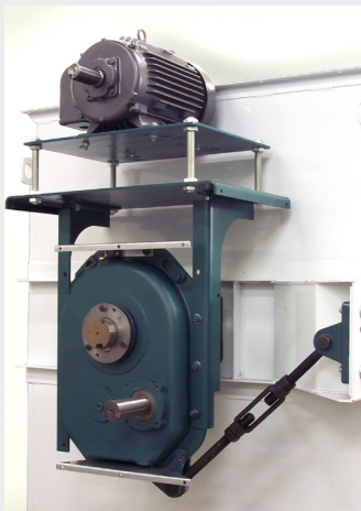
Torque arm reducer drive. Belt guard is removed for illustration purposes
