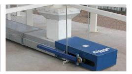
For maximum efficiency, the bottom of the tank outlets should be level with the outer top edges of the belt or extend to ½" below the edges.
