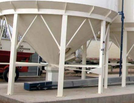
CONVEYORS CAN BE MOUNTED ON STANDS OR SUSPENDED FROM HOPPER BINS.
