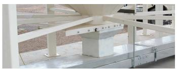
12" square transitions make quick tank-to-conveyor connections.
