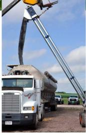
Can be installed horizontally or at an incline up to 60° and doesn't necessarily require a catwalk support system like a traditional conveyor might.
