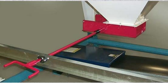
The rack & pinion gate has an extended control rod for easy operation.
