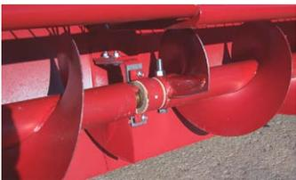
The 5/16 flighting runs on oil-impregnated wood block hanger bearings.
