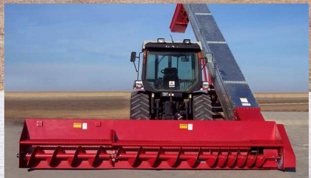
The Ultra Scoop features a 16 foot wide scoop with a 6 foot detachable wing that folds for legal highway transport.
