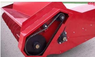
Chain drive is designed for strength and simplicity.
