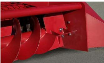
A heavy duty 4-blade "flapper" at the transition to the incline conveyor force feeds the conveyor for maximum capacities.
