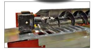
Heavy Duty Double Gearbox Sweep Drive Internally controlled engage/disengagement for the sweep auger. The gearboxes are oilbath types with 1¼" shafting.
