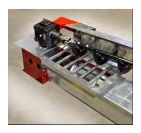
**Center Sump**UHMW pads provide easy gate movement.
