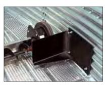
**Sweep Stop** - Limits the sweep to one revolution. The Stop swings back, allowing the Sweep to be moved forward over the sumps before refilling the bin.
